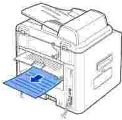
Printing from the manual feeder to the rear output slot provides a straight paper path. Using the rear output slot might improve the output quality with the following:
